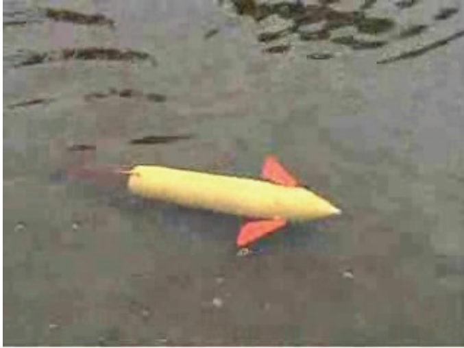
Fig. 34. Prototype was investigated in a large storage lake with autonomy power pack and distance control system, moving in real under water conditions with waves
