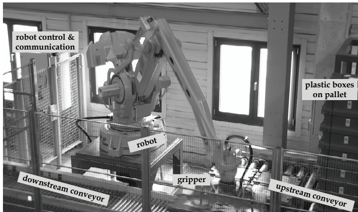
Fig. 9. Industrial application of a robotic system for depalletizing plastic boxes: result of the ontological configuration [source: author's illustration]
