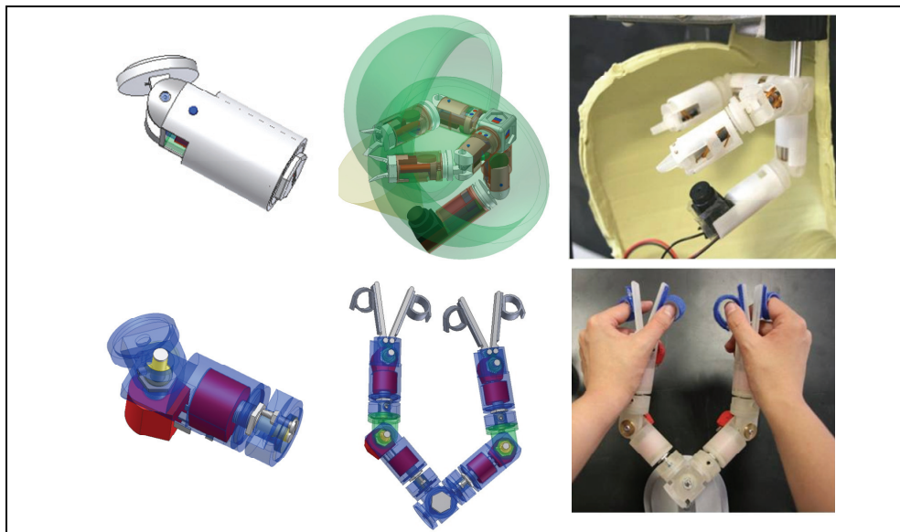
Fig. 6. Robotic modules (top line) and the reconfigurable master device (bottom line): one module (left), assembled modules (middle) and prototypes (right)
