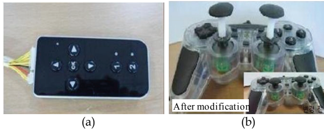
Fig. 16. Input devices of a self-feeding robot. (a) Buttons, (b) Joysticks
