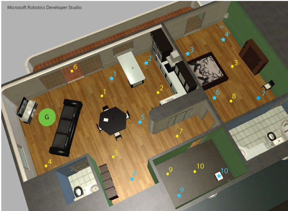
Fig. 1. Simulation Environment (Microsoft, 2011) used for evaluations. Blue stars and yellow dots represent starting positions used for demonstrations and test runs, respectively. The green area marked with a G represents the target position. The white area under star 10 is the robot.
