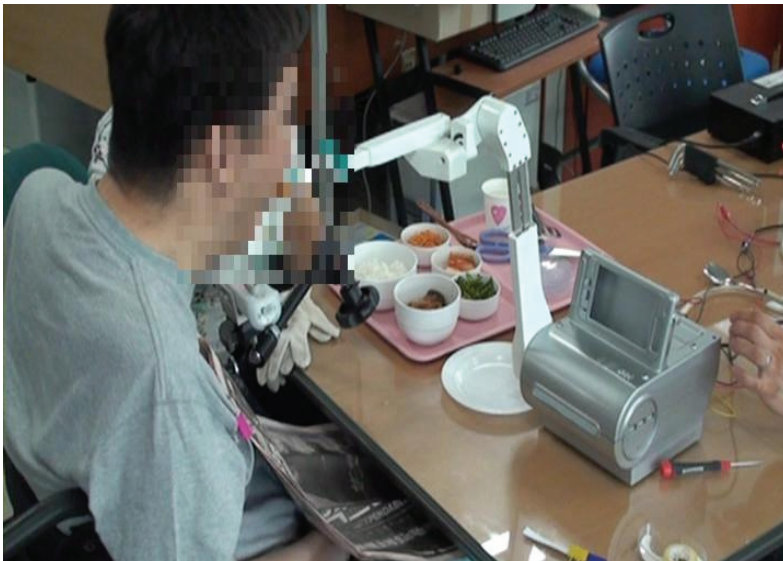
Fig. 14. The motions of the self-feeding robot in single-arm configuration. The caregiver picks food up on the spoon of the self-feeding robot, and then the user presses the button to receive the food
