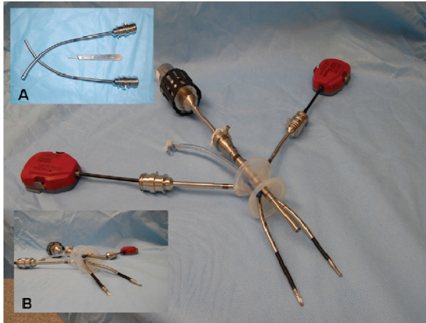
Fig. 5. VeSPA instruments and accessories. (A) Curved cannulae; (B) multichannel single-port, 8.5-mm robotic scope, flexible instruments passed through the cannulae
