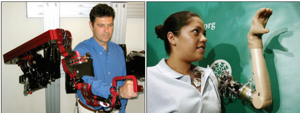
Fig. 1. (Left), orthotic robot of upper parts (Perry et al., 2007). (Right), prosthetic robot of upper parts (Rehabilitation Institute of Chicago, 2006)
