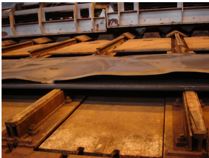
Fig. 1. Picture of poor strip produced during hot rolling.
