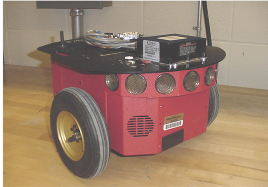
Fig. 4. The mobile robot with gyroscope.
