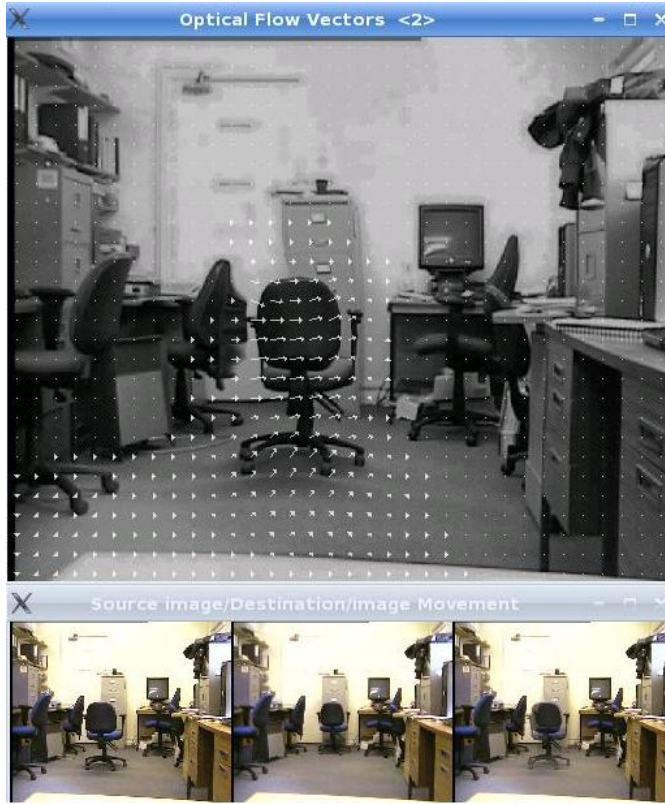
Fig. 1. Optical Flow vectors (Guzel & Bicker, 2010).
