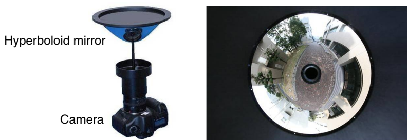
Fig. 1. Omnidirectional camera equipped with a hyperboloid mirror. The left figure shows an acquired image.
