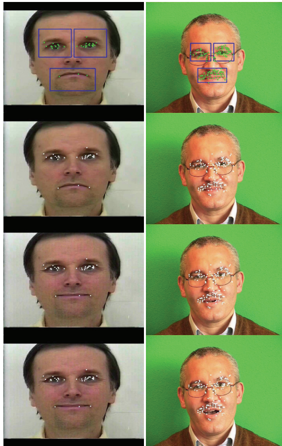
Fig. 12. Extraction of feature points in the bounding box for the first frame and Feature points tracking using pyramidal Lucas-Kanade in the remaining of the sequence.
