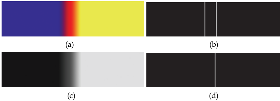
Fig. 8. Pixels of adjacent different colored objects with strictly monotonous gray level values. (a) color image. (b) color declivity image. (c) the corresponding gray level image of (a). (d) declivity image.
