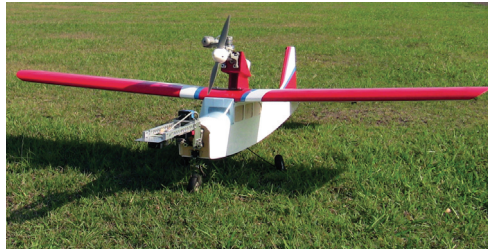
Fig. 7. The aircraft used for flight testing was a Super Frontier Senior-46 (wingspan 2040mm), modified so that the engine and propeller assembly is mounted above the wing.
