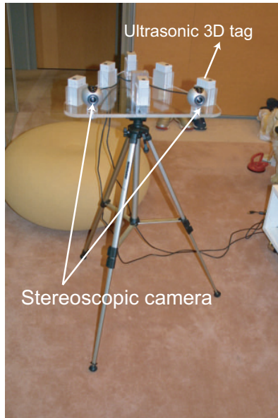
Fig. 24. UltraVision (a stereoscopic camera with the ultrasonic 3D tags) for creating simplified 3D shape model
