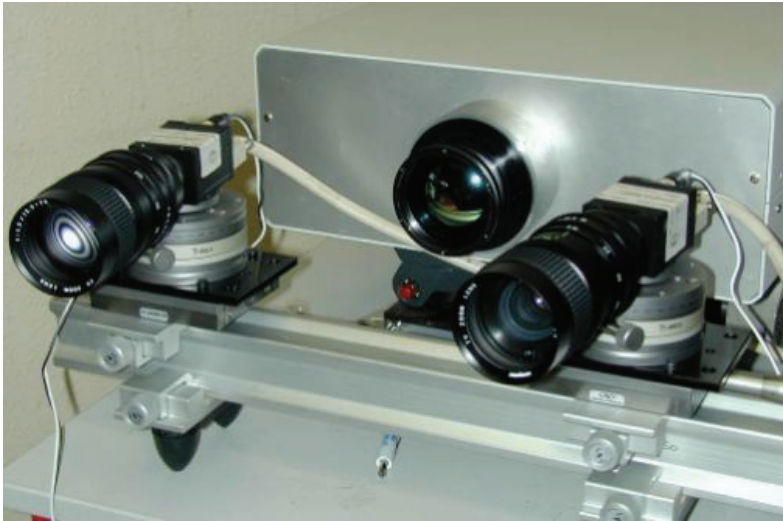
Fig. 18. Three cameras (the central FIR) connected to the computing unit.
