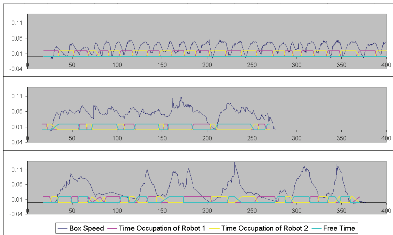
Fig. 5. The time distribution curves for teleoperation (upper) and waypoint control (middle) for homogeneous robots, and waypoint control (bottom) for heterogeneous robots
