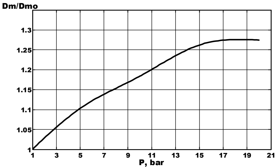
Fig. 20. The dependence of relative size of droplets in spray behind injector on combustion-chamber pressure.
