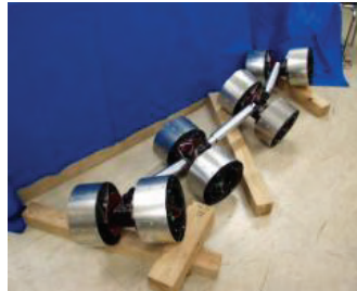
Fig. 7. Robot Genbu representing group of active wheels – passive joints robots
