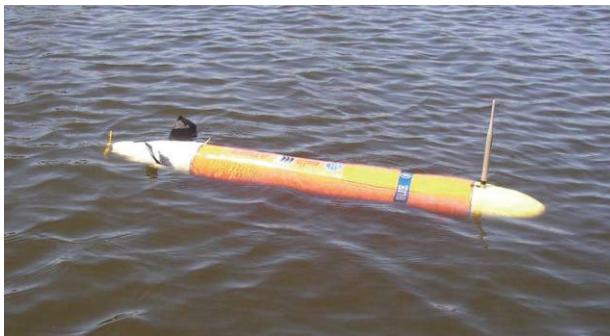
Fig. 1. Light Autonomous Underwater Vehicle (LAUV) designed and built at University of Porto.
