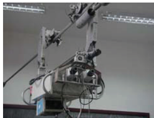
Fig. 19. The cable-climbing robot presented in (Fu et al., 2006)
