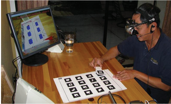
Fig. 10. A participant using the AR-HRC system. The image on the monitor is what is being displayed to the user in the HMD.
