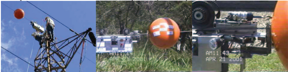
Fig. 10. The aircraft warning sphere installation and removal mechanism proposed in (Campos et al., 2002)
