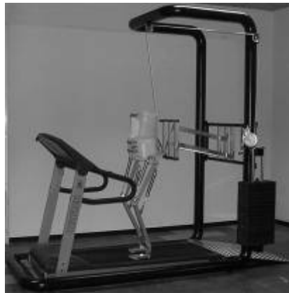
Fig. 5. Realized prototype of the overall rehabilitation system
