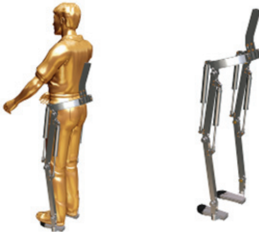
Fig. 4. Mechanical ergonomic structure of the exoskeleton with pneumatic actuators
