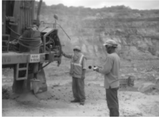
Fig. 15. Sound measurement during drilling
