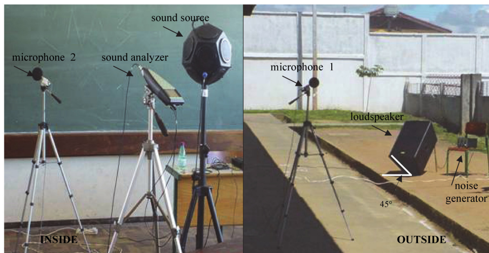
Fig. 2. Measurement of façade insulation according to ISO 140-5 10
