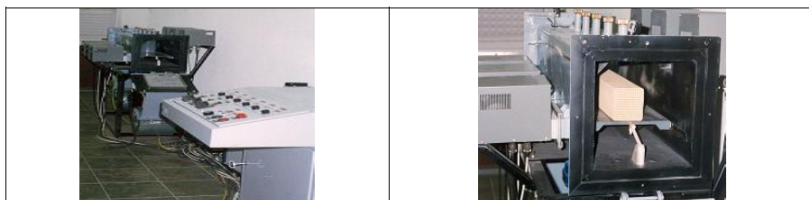
Fig. 5. Drying of creaming carrier in a microwave dryer.
