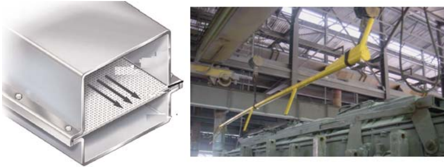
Fig. 18. The Albras aluminum smelter air fluidized conveyor and a conventional air slide in the left.
