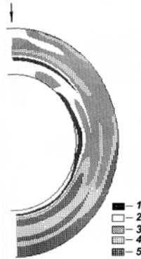
Fig. 10. Distribution of the relative heat transfer coefficient over the surface of type 2 fin ( h/d = 0.357 ) located in the frontal row of the bundle. Re = 2 \cdot 10^4 ; the free-stream direction is from the top down. a_i/a_{av} : 1) 1.94 to 1.66; 2) 1.66 to 1.24; 3) 1.24 to 0.83; 4) 0.83 to 0.41; 5) 0.41 to 0.11
