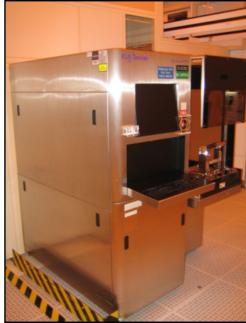
Fig. 11. The SP1 machine which measure the particle
