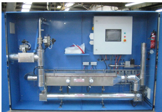
Fig. 5. Catalytic pilot reactor at final completion (Catalytic Solutions International Pty Ltd - Australia, 2011).
