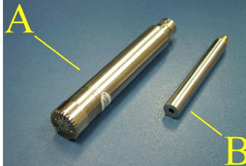
Fig. 5. Preamplifier for condenser (A) and electret (B) microphones (microphones attached)
