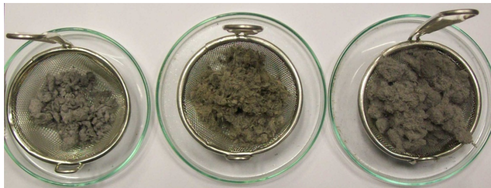
Fig. 5. Raw PMS (left), unraveled PMS (middle) and fluffed PMS (right).
