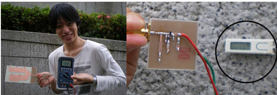
Fig. 16. Directly powering a thermometer mounted on a car park wall (right picture). The maximum instant voltage rectification on record equals 3.7 V (left picture).
