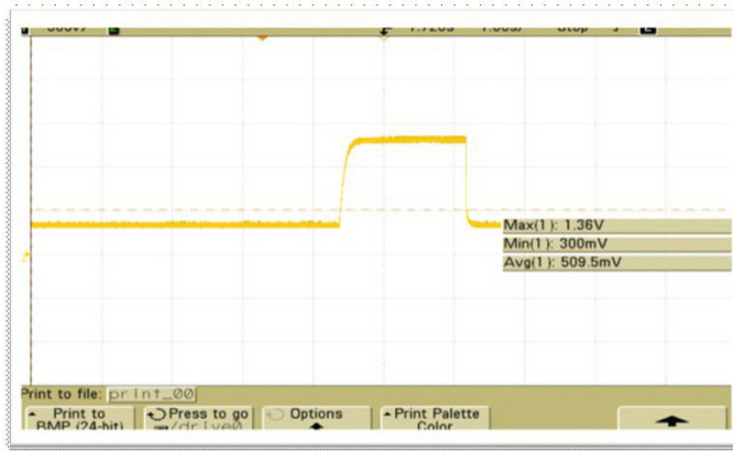
Fig. 13. Voltage across PV panel
