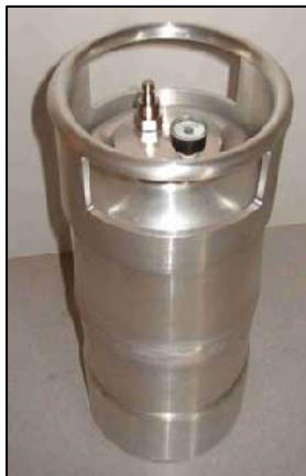
Fig. 5. Hydrogen storage reactor containing LaNi 4.7 Al 0.3 alloy with a capacity for 1500 NL H 2 .
