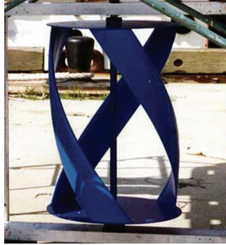
Fig. 12. Gorlov turbine (Source: http://www.oce.uri.edu/oce311/ )
