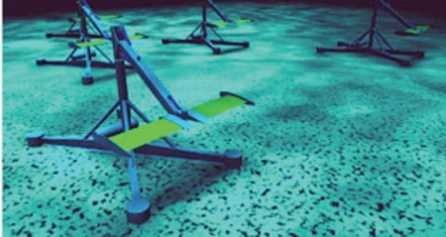
Fig. 16. Stingray tidal energy conversion device using oscillating hydroplane (Source: http://www.engb.com/services_09a.php )
