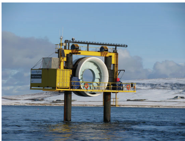
Fig. 7. Open centre tidal turbine (Source: http://www.greentechmedia.com/articles/photos-clean-power-at-the-edge-of-the-world-5723.html )
