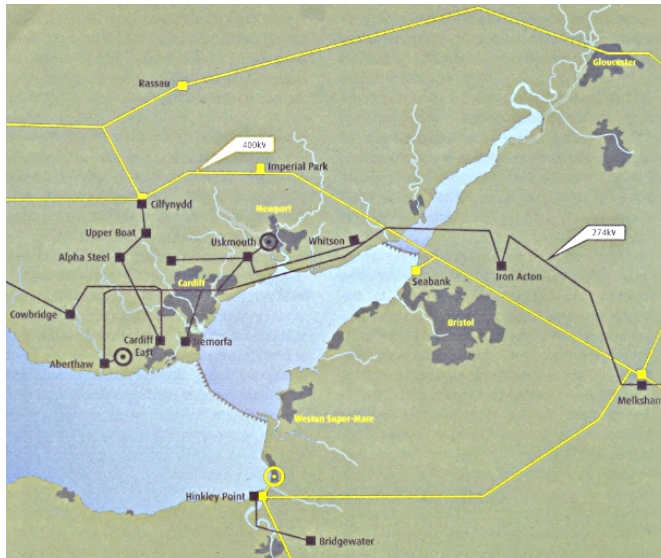
Fig. 14. Electricity Transmission Network (400 and 275kV) around the Severn Estuary.
