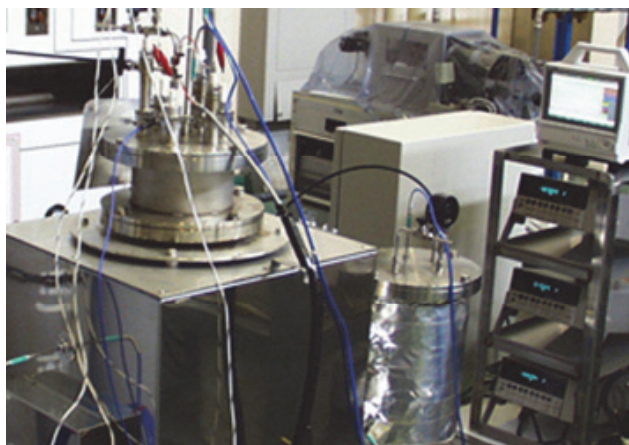
Fig. 9. Photo of the comparison apparatus of oxygen sensors. Three sensors can be compared in liquid LBE.
