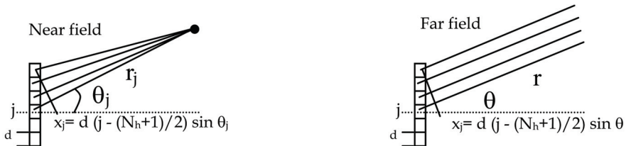
Fig. 18. Equally spaced linear array of hydrophone elements being intercepted by a propagating wave front at beam angles \theta_j for the near field configuration (left) with beam angle \theta for the far field (right) approximation.
