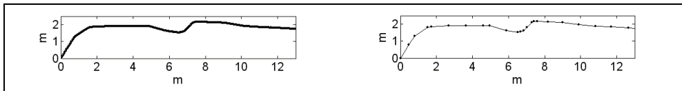
Fig. 5. Fragment of a real trajectory (left) and the polyline that approximates it (right). The dots represent the vertices.
