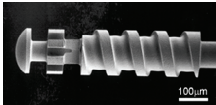
Fig. 3. A sample stainless-steel 3-D structure machined using a 5-axis \mu EDM system.
