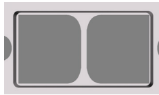
Fig. 3. Schematic of a silicon carbide tensile specimen in a silicon support frame
