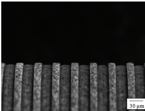
Fig. 15. SEM image of coil lines by chemical etching.
