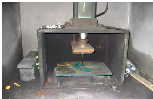
Fig. 1. Nail penetration Test equipment.
