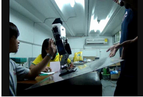
Fig. 12. Robot Inclined Steel Plate Balancing Experiment. Back position. Note that the hand of the person is not touching the robot. This is just in preparation to catch the robot when it falls.
