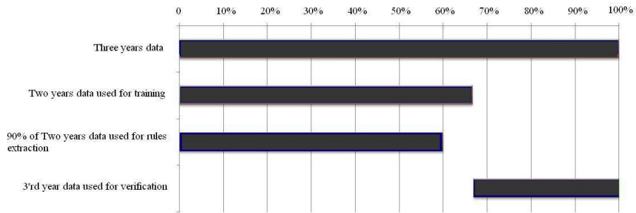
Fig. 5. Modelling data utilization for the ECU’s Joondalup Campus energy consumption
