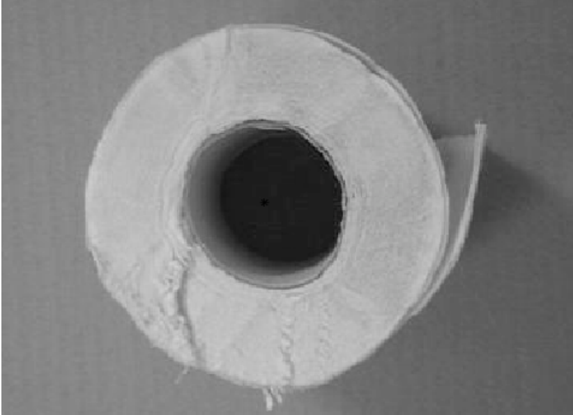
Fig. 8. Defects on the roll surface.
