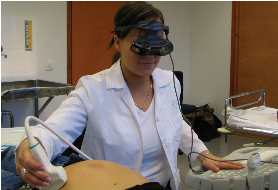
Fig. 3. Ultrasound scanning with the see through biocular display. The midwife can see the ultrasound scanning image in her visual field and simultaneously follow the location of the probe through the see-through display.
