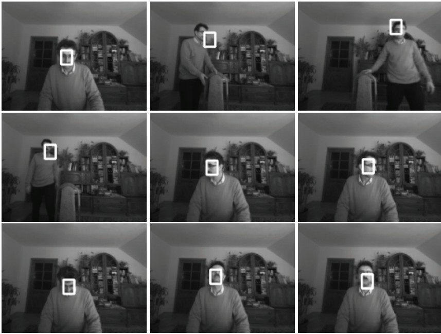
Fig. 6. Face tracking using multi-part object representation in case of occlusions. Frames #1, #15, #25, #45, #46, #48, #55, #65, #70 (from left to right and from top to bottom)
