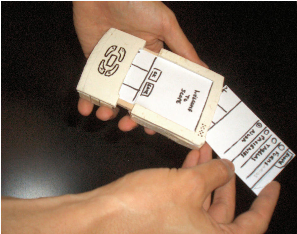
Fig. 2. Low-Fi prototyping frame mimicking a Palm T3 Tungsten. The slot allows users to easily exchange cards/sketches).
