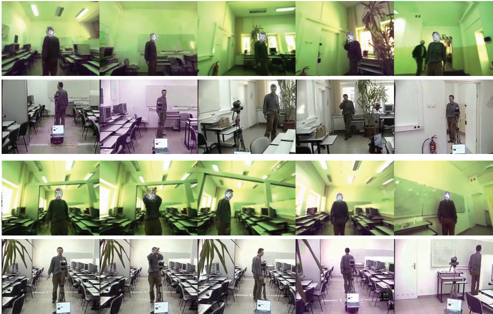
Fig. 2. Person following with a mobile robot. In 1-st and 3-rd row some images from on-board camera are depicted, whereas in 2-nd and 4-th row the corresponding images from an external camera are presented
