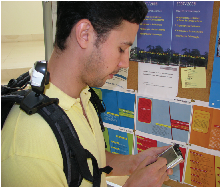
Fig. 5. Mobile video evaluation kit. The camera attached to the user's shoulder captures video footage of his interaction with the device/application.
