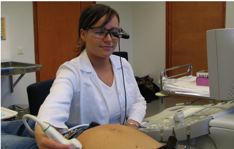
Fig. 2. Ultrasound scanning with the monocular display. The midwife can see the ultrasound scanning image in her left visual field and simultaneously follow the location of the probe with both eyes.
