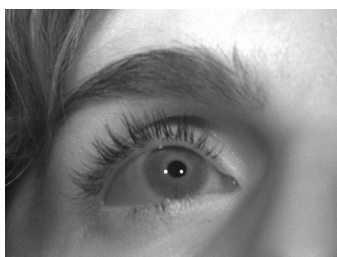
Figure 1. Image of the eye captured by the camera. The corneal reflections are the bright dots in the image
