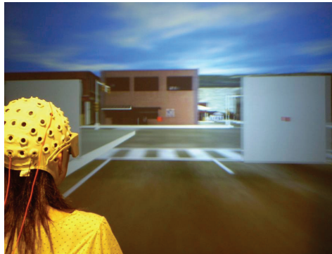
Figure 2. The left and right flickering (white/black) visual stimuli with square shape superposed on a front screen and a subject sitting in immersive virtual environment. These two flickering frequencies have different rates
