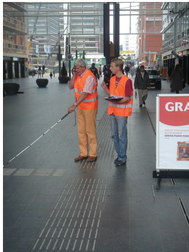
Figure 4. A visually impaired pedestrian explores the different routes on the crossing point of the guideline during the test
