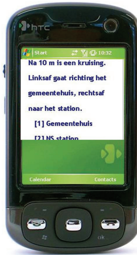
Figure 5. An example of a Smartphone to use ASK-IT to guide visually impaired pedestrians in The Hague
