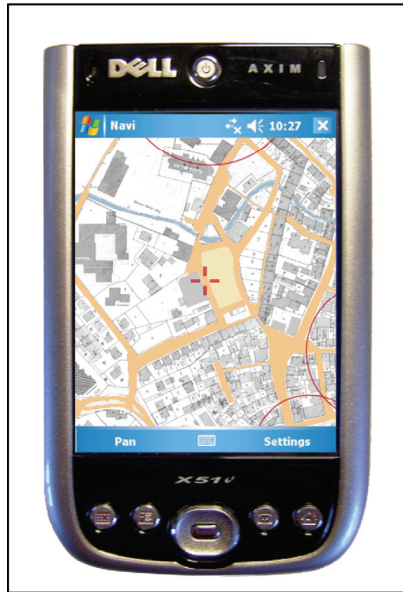
Figure 7. A context aware application using Halo circles to show off screen locations (Mahler et al. 2007)
