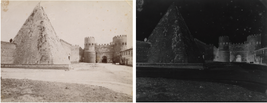
Figure 2. Original Pyramid image ( Left ) and its Saturation component ( Right ): blotches are more visible in the Saturation component and appear as bright regions
