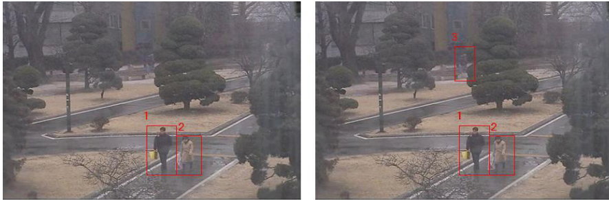
(a) Object detection using shape information (b) Object detection using shape and motion information
