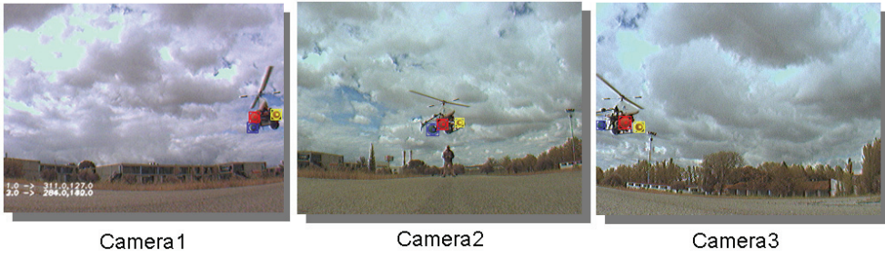
Fig. 4. Feature Extraction. Different features must be extracted from images taken by different cameras. In this example color-based features have been considered.
