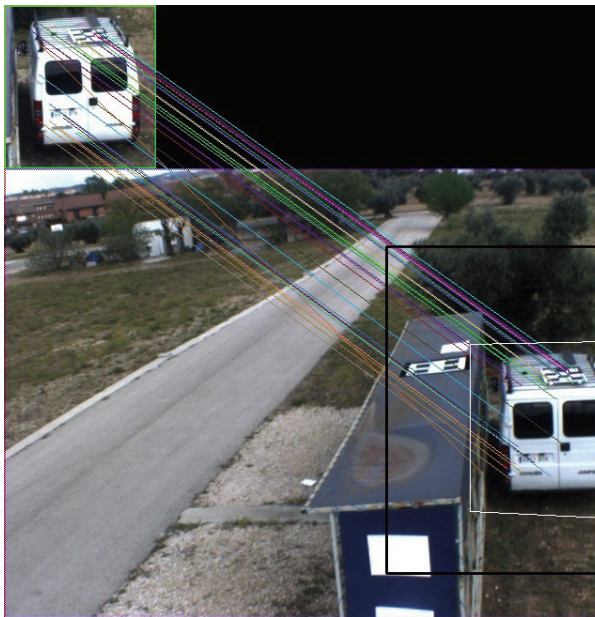
Fig. 2. Robust Homography Estimation using SURF features on a car tracking from a UAV. Up: Reference template. Down: Scene view, in which are present translation, rotation, and occlusions.
