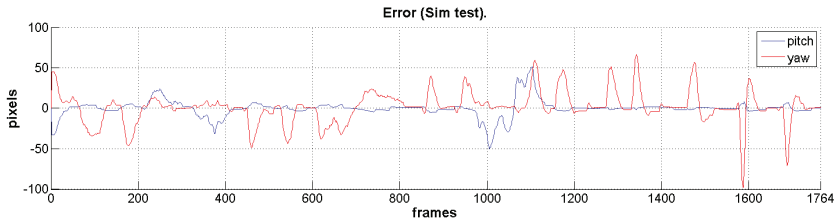
Fig. 27. Error between the static object tracked and the center of the image, running with the UAV simulator.
