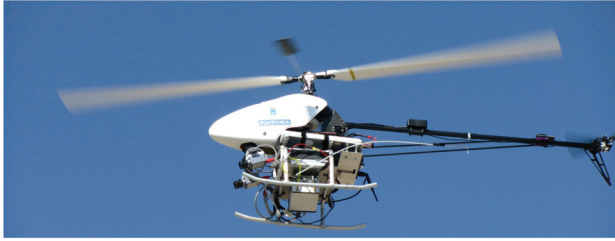
Fig. 14. COLIBRI III Electric helicopter UAV used in a dynamic look-and-move control architecture.
