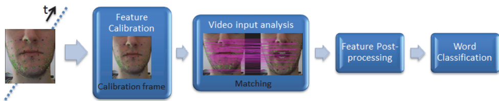
Fig. 6. The phases of our Visual Speech Recognition experiment.
