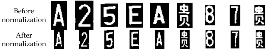
Fig. 3. Character images before (upper) and after(lower) size normalization
