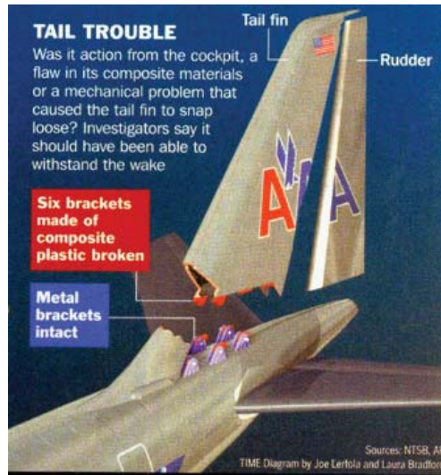
Figure 6.23 Illustration of the aircraft tail section failure at the November 2001 crash (source: TIME, November 26, 2001)
